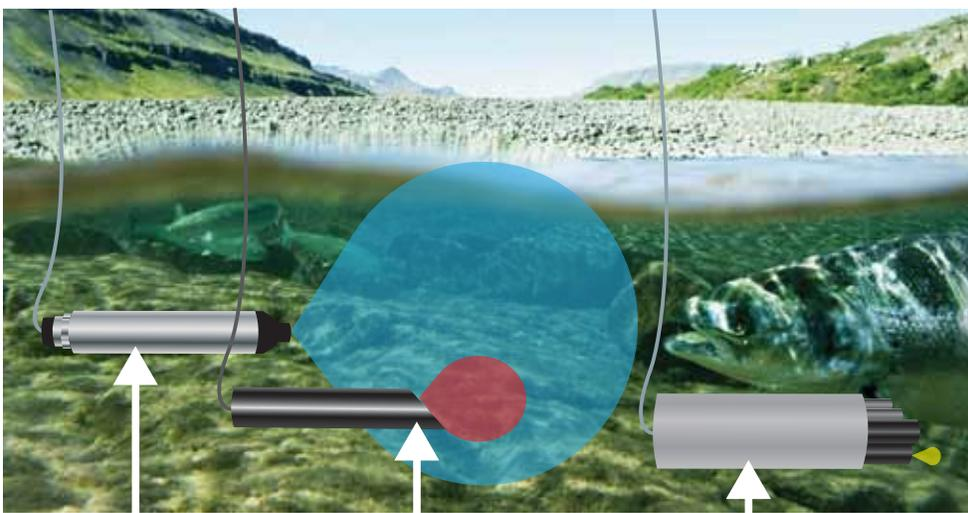
Typical single-parameter sensor has a large viewing volume that often intersects the surface and riverbed, generating false turbidities.
