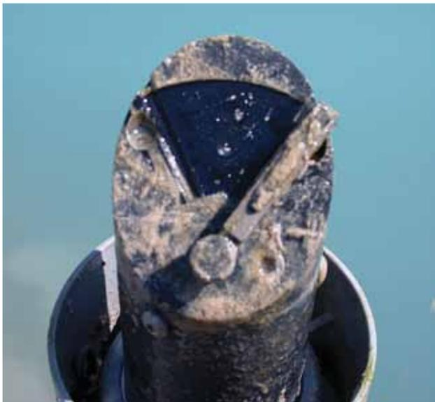
Despite significant bio-fouling after a 12 month deployment, the optical face of the DTS-12 is clean and perfectly operational.
