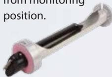
Connect the DTS-12 directly to an ISCO automatic water sampler with an ISCO interface cable.
